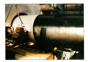
Pipes being coated with three layer side extruded high density polyethylene external coating
