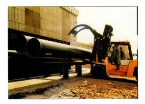
Precoated pipes from the outgoing racks being transferred to storage area.
