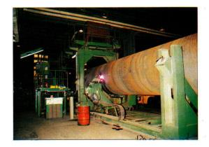
Pipe being cut outomatically at the plasma arc cutting station.
